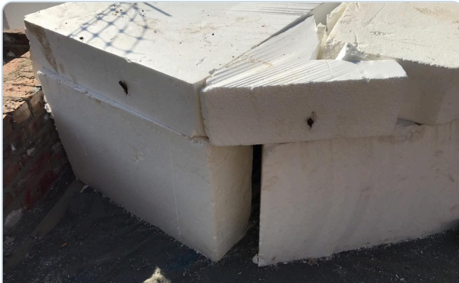
True scale — a single 2550 × 1250 × 960 mm block, cut and shaped on site with a saw.
