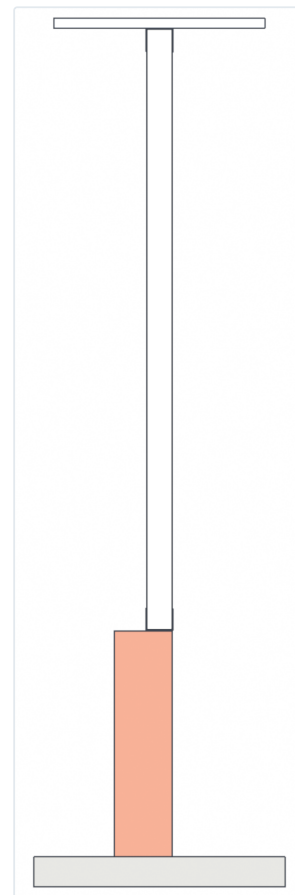
The whole wall: slab, dwarf wall, channel, panel, head cap, ceiling over.
