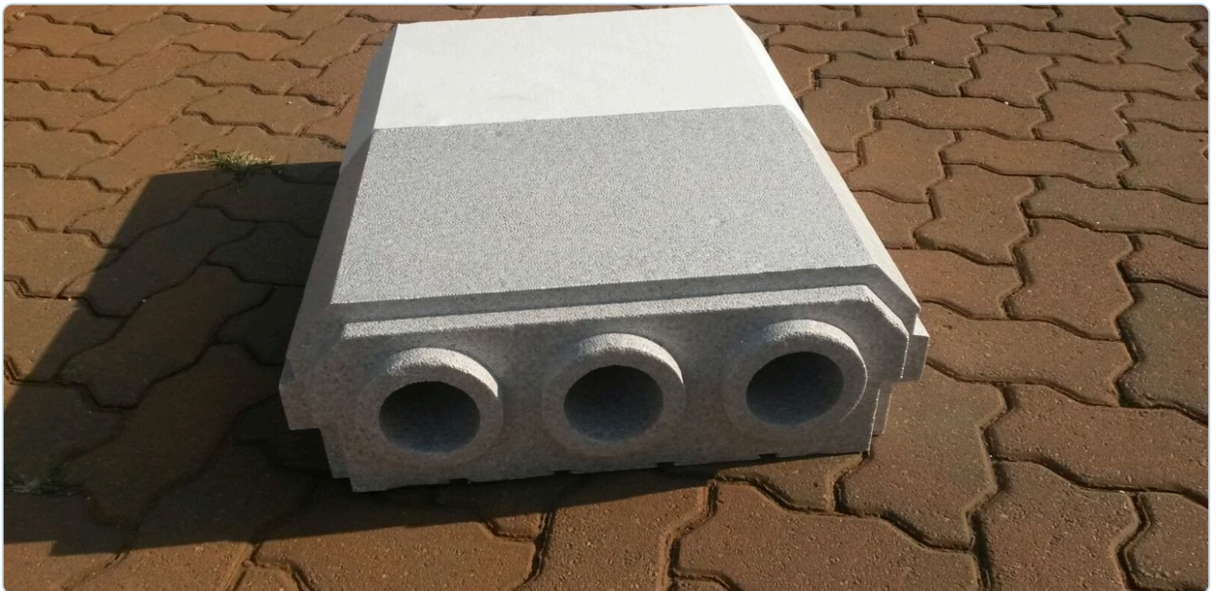
Technoblock #190 — moulded flame-retardant EPS block with three longitudinal cores, laid between pre-cast concrete ribs in place of cement blocks.
